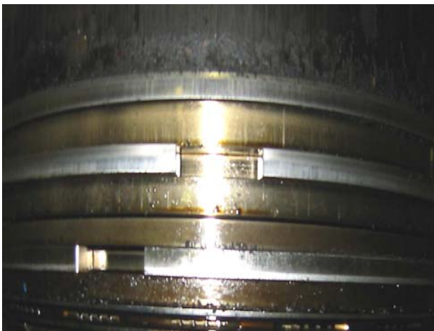
Figure 1 Clean piston 4000 hours of Salyx TBN 50 application in engine with heavy fuel (1.5 - 5 % wt Sulphur content).
